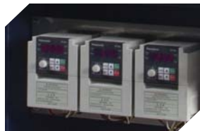
Inverter array for synchronization
